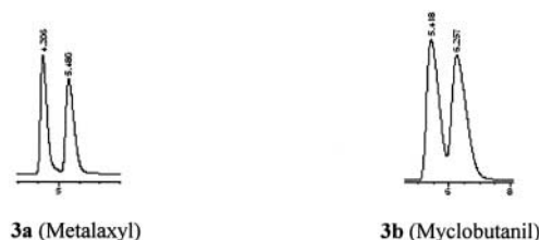
Figure 3. The chromatograms of pesticides in acetonitrile/water (70 : 30 v/v, flow rate is 0.8 mL/min, room temperature).
